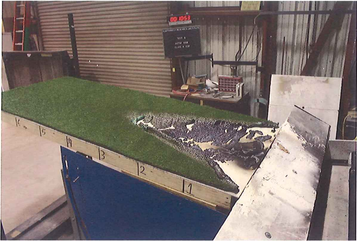
Figure A-3. Sample at the end of the flame exposure.
